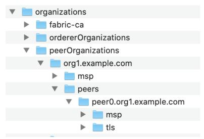
The figure above shows the subfolders inside of a peer owned by the organization. Note the msp folder here under the peers folder. This is the local MSP of the peer, not a duplicate of the org1.example.com MSP.
